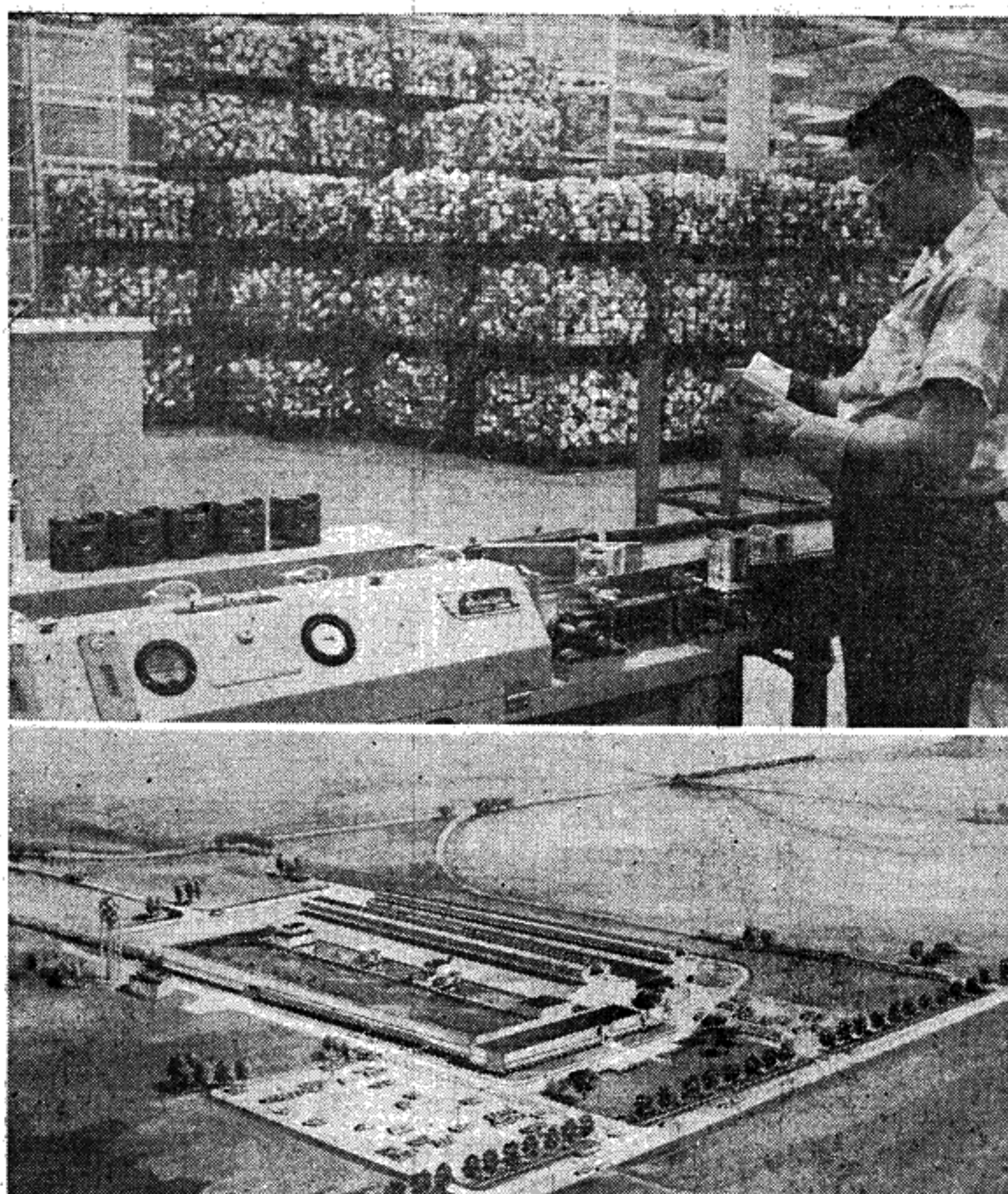
Lower picture shows Ford Motor Company Aluminum Castings plant at Sheffield, Alabama. Upper photo: Engine pistons moving by conveyor through automatic weight checker. Castings also are visually checked before shipment.
