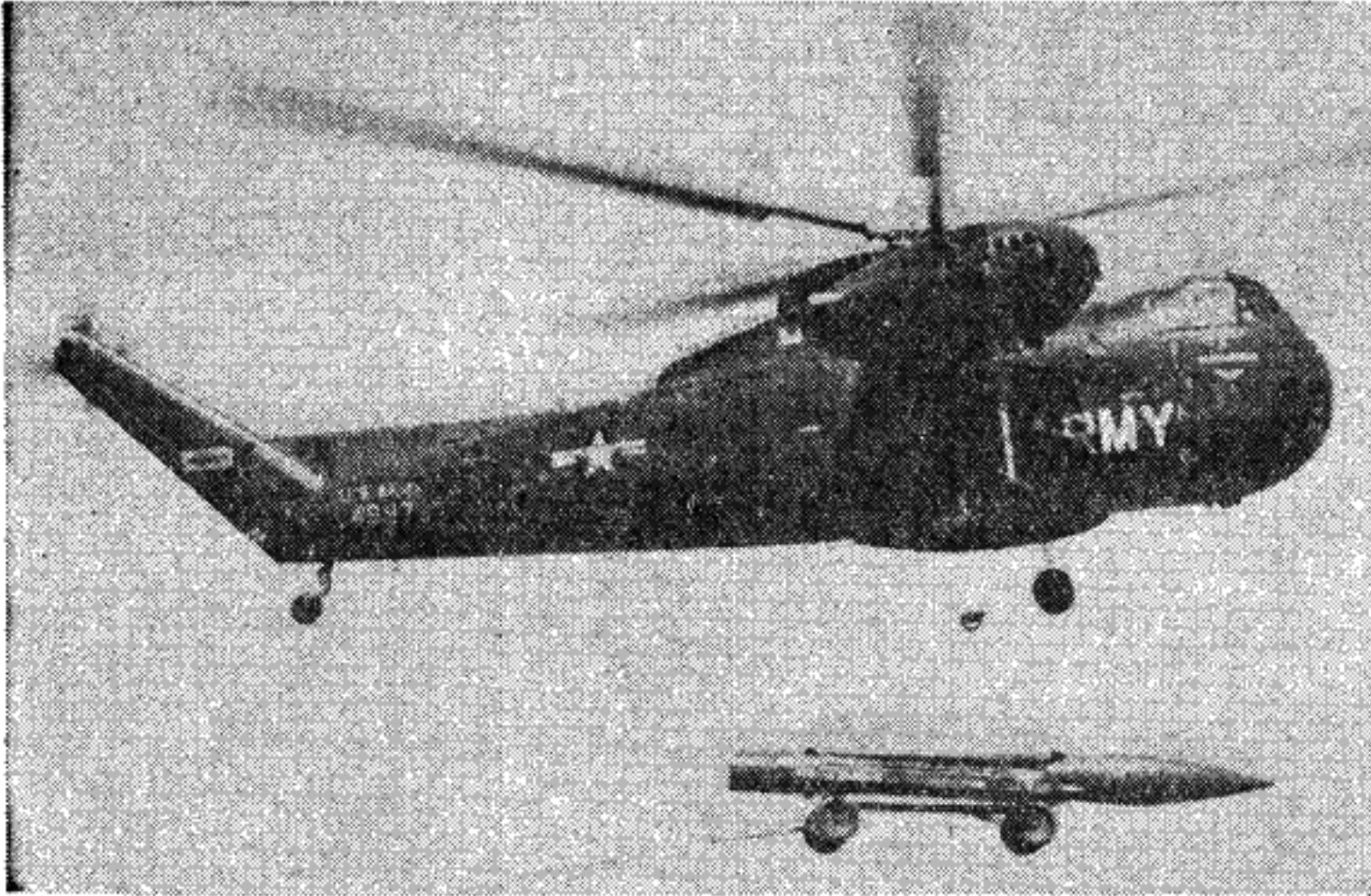
CHOPPER JOHN —The world's largest production helicopter, the Army's Mojave, carries an Honest John rocket and special launcher in a sling in a mobility experiment. As publicly demonstrated at Fort Bliss, Tex., recently, the Honest John is normally fired from a truck.
